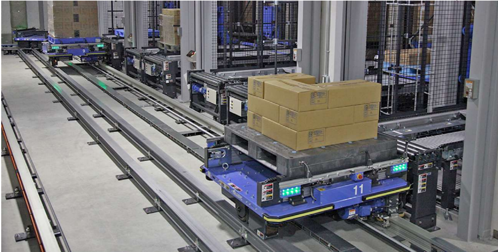
Automated transportation & sorting vehicle – the rail-guided carriage system transports heavy-duty pallets at high speed.
