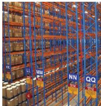
Narrow aisle pallet racking
